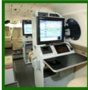
*The NTP's Airborne Navigation Trainer aboard a RAAF B300 King Air aircraft.*
