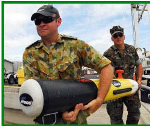
Hydroid REMUS 100 Autonomous Underwater Vehicle to be operated by the Royal Australian Navy
