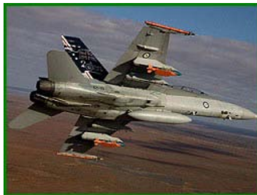
A Royal Australian Air Force F/A-18 Hornet in flight with two JDAM-ER 500lb bombs and two Time Space Position Information pods.
